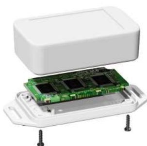
A 1.6 mm thick PCB can be clamped directly between the enclosure parts and optionally hot melted and clenched via two pins.
