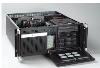
Easy-to-maintain system fan & reusable filter design
